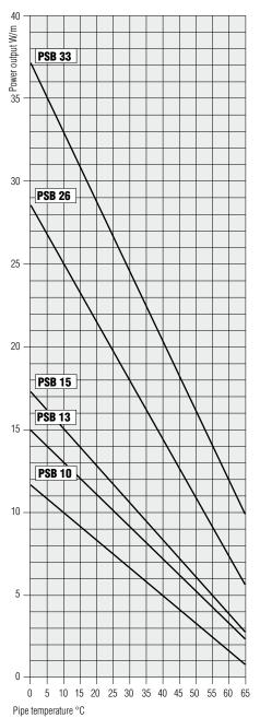
Power output on insulated steel pipes at  ${\bf 230~V}$  under nominal conditions.
