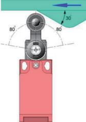
The actuating cam should be profiled at 30° for optimum operation. (Plunger-type switches operate from a flat profile.)
