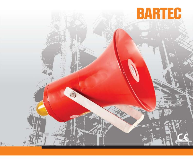
BHB150-1 series Ex Sounder & Beacon is designed according to ATEX and IECEx standards. Enclosure material is UV and corrosion resistance GRP (Glass Reinforced Polyester). This product is certified for use and installation in Zone 1 and Zone 2 areas with gas groups IIA, IIB, IIC and temperature class T4-T6. It specially applies to Oil & Gas, Offshore Platforms, Chemical, Petrochemical, Refinery and Marine Industries.
