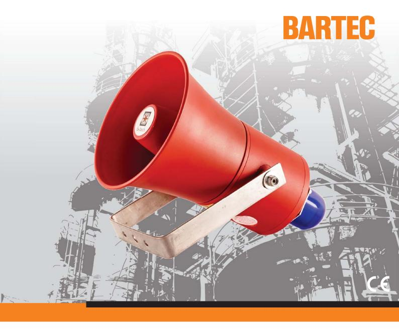
BHB125-1 Ex Sounder & Beacon is designed according to ATEX and IECEx standards. Enclosure material is Stainless steel. This product is certified for use and installation in Zone 1 and Zone 2 areas with gas groups IIA, IIB, IIC and temperature class T4-T6. It specially applies to Oil & Gas, Offshore Platforms, Chemical, Petrochemical, Refinery and Marine Industries.
