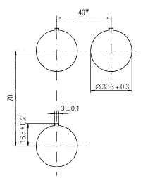
\* Recommended distance for mushroom pushbutton, emergency switch as well as position selector with protective shroud: 100 mm.
